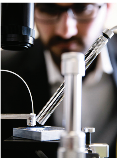
Left | middle: R&D project with Bodle Technologies to laser construction information almost invisible to the eye on the surface of a glass panel. Crucial information about the type of glass, composite, coatings, frits, when and where it was made will aid demolition contractors to reuse or recycle the glass
