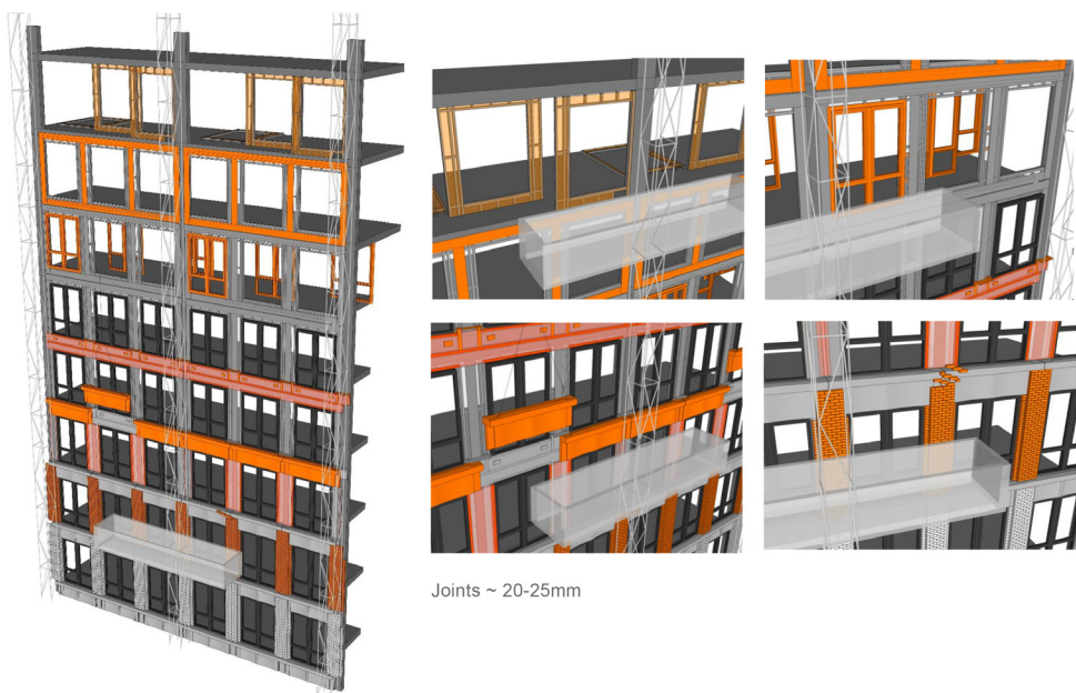
Hand laid brick with precast rainscreen
